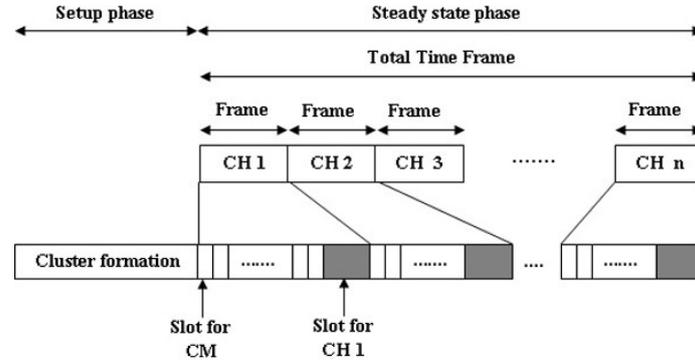
Fig. 1. Time slot structure of EDCGRP.
