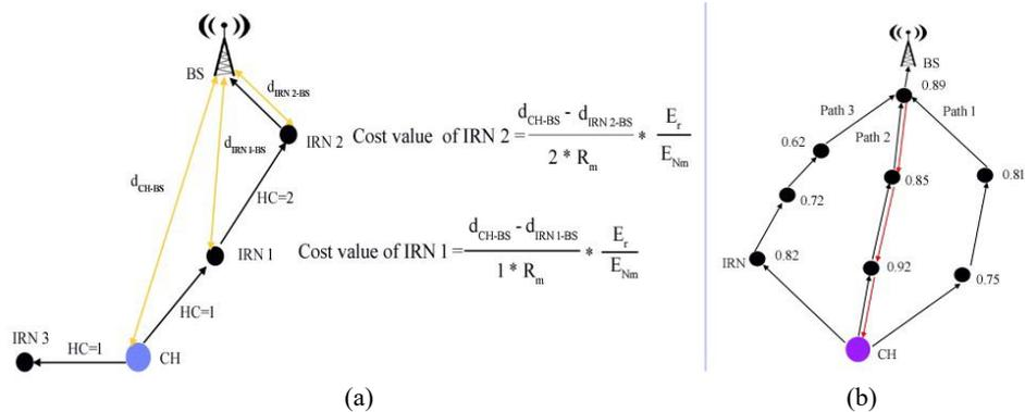
Fig. 3. (a) Selection of IRN; (b) Example for gradient based on-demand routing.
