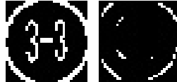
Fig. 2. Detected circle (left) before and (right) after removal of the inside objects.
